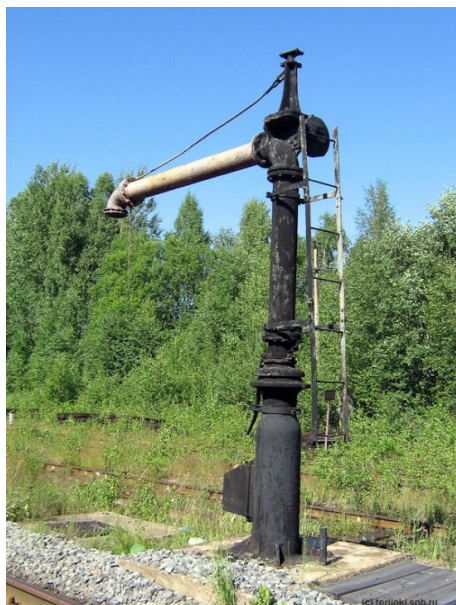
Pic. 9. Column position in non-working condition.
